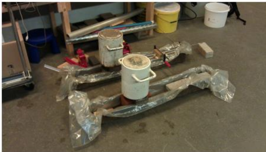
Figure 11.9: Two set-ups of the horizontal shear test
